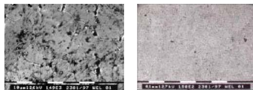
A magnification of 1500x shows a significant amount of dirt in the pores on the surface and this, in itself, should not be considered an exception. In fact, this is more the rule than an exception.
