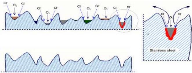
Above is a diagrammatic representation of a stainless steel surface that has greatly been magnified. The pores are filled with all kinds of dirt deposits, under which chlorides will find it easy to move. This will be much easier for small chlorine ions than for relatively large oxygen molecules and that is precisely the problem. Chlorine, just like fluorine, iodine and bromine, is a member of the halogen family, which are known as salt formers. Chlorine ions will therefore
